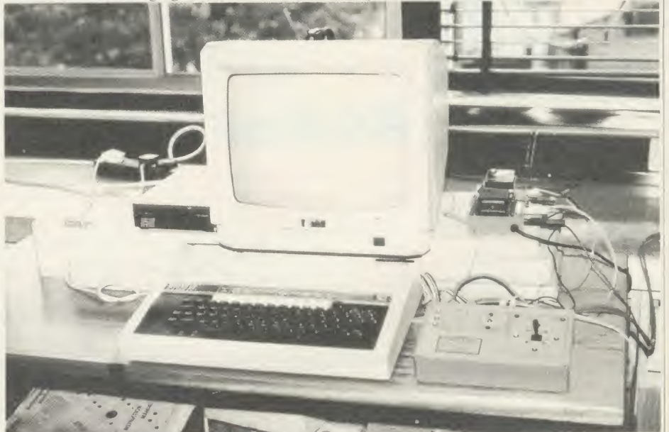
Antenna control station: BBC micro and control box
